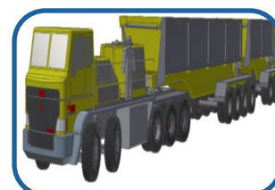
400T + Electric Drive Road Train
